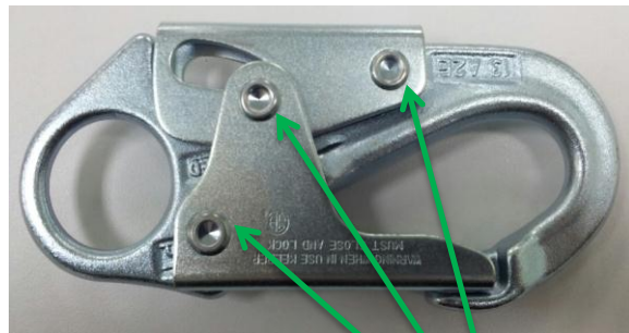
Rivet in Place
